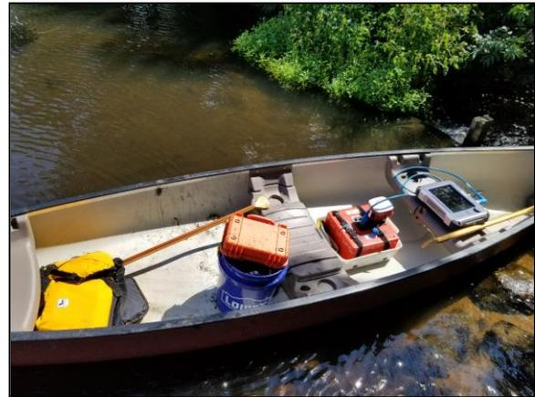
*GPR collection setup, with flat-bottom canoe, GSSI 400 MHz antenna and SIR 4000 tablet.*
